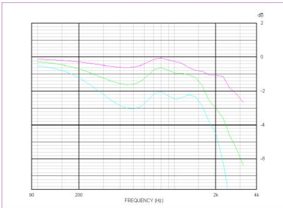
Figure 8. Off-axis response of a piston in R109 uni-Q cabinet. The curves are the acoustic pressure response at 15, 30 and 45 degrees horizontally off-axis, all relative to on-axis.
