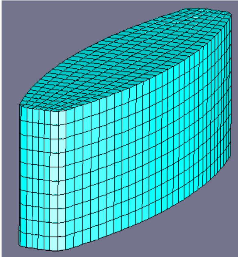
Figure 7. Finite Element Model of the Uni-Q enclosure.
