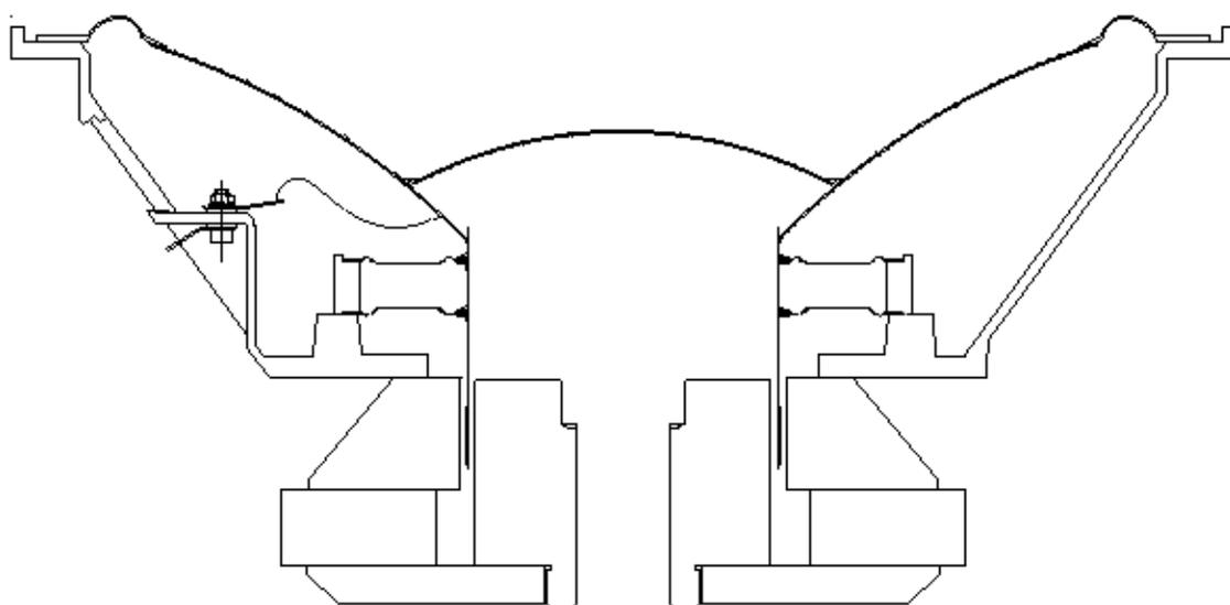
Figure 2. Cross-section of the new SP1405 Low Frequency Unit.
