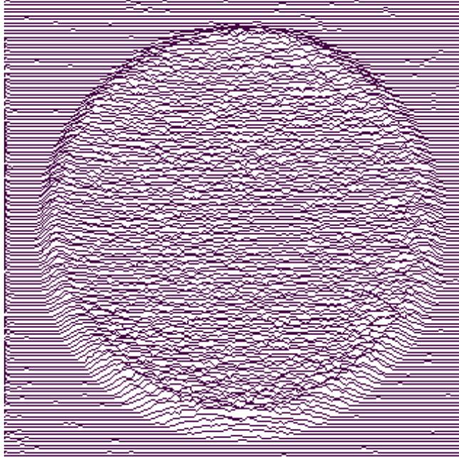
Figure 3. Laser scan of the SP1405 bass unit at 300Hz. The slight deformation of the surround is the first indication of non-piston behaviour, this is well above the crossover point of 100Hz.
