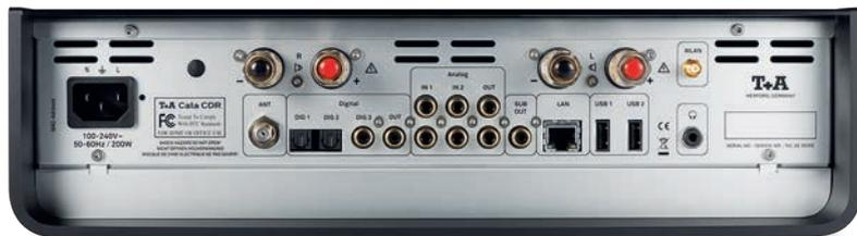
**ABOVE:** Coaxial, optical (x2) and USB digital inputs are joined by wired and wireless LAN, two USB-A (HDD), FM/DAB radio and two RCA/XLR line inputs. A coax digital out joins preamp/sub line outs, a 3.5mm headphone port and 4mm speaker terminals
